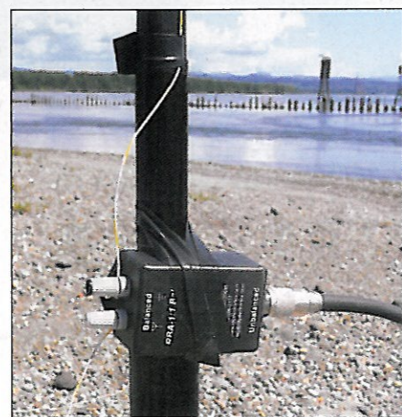
Figure 2 — Detailed view of the antenna feed connections. Vinyl electrical tape is used to secure the wire, pole sections and commercial 1:1 balun.
