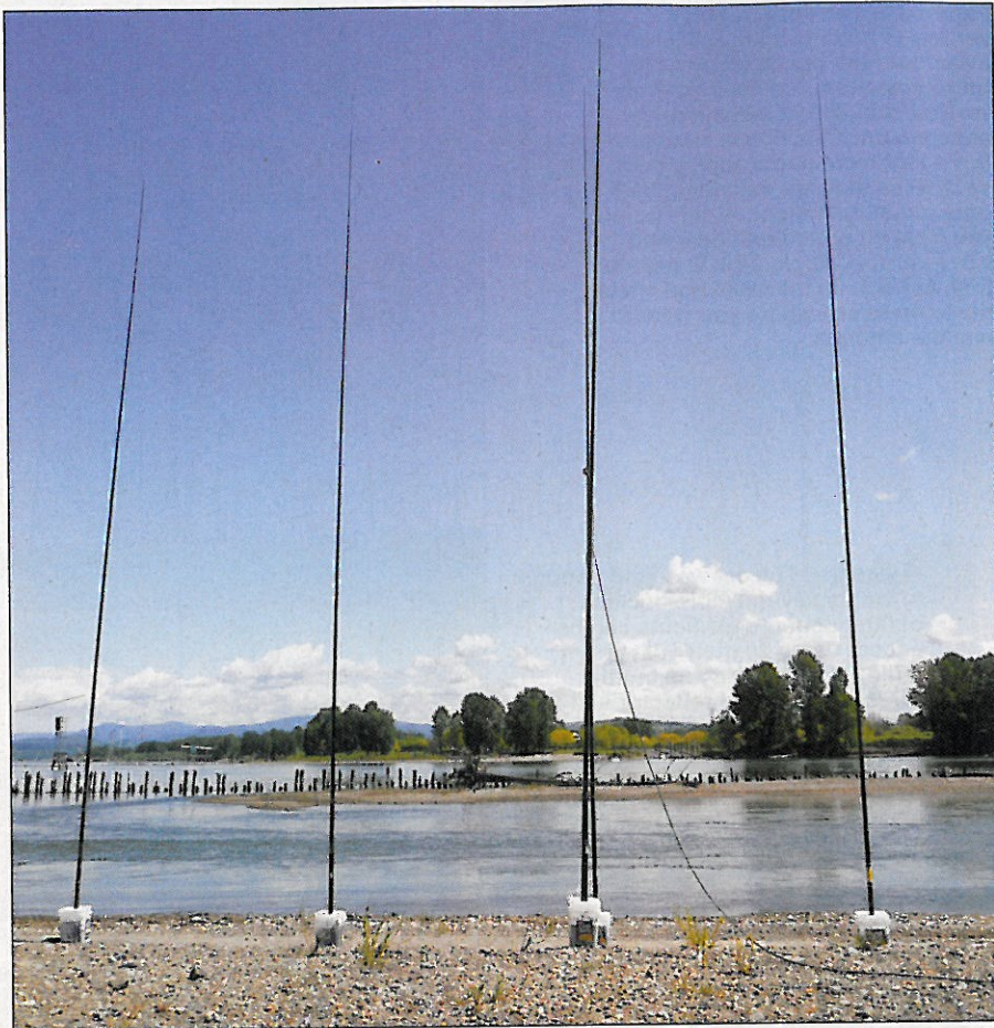
Figure 6 — Side view of the four element 20 meter Yagi deployed on the beach on McGuire Island in the Columbia River.
